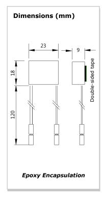
For coils with power < 80W Voltage 0 ... 24Vdc Weigth 6g
