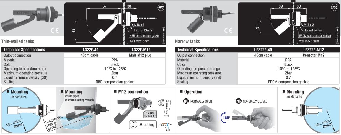
Constructive materials PPA Polyphthalamide (High mechanical and temperature resistance) PA Polyamide (hex nut) Electrical contact: reed switch 20W/VA;
